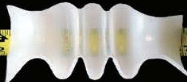
Severe thinning is evident by the translucency of the convolutions above. Permanently yielding (stretching) PTFE beyond its elastic limit will compromise the materials mechanical integrity and can cause sudden premature failure.
