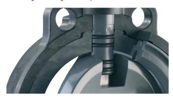
The shaft, disc and face seals all operate independently from one another. This eliminates issues common to booted style centric valves such as crimping, where the compression of the valve between two flanges causes the boot to ripple. This can lead to increased operating torque and wear, ultimately reducing the useful life of the valve.
