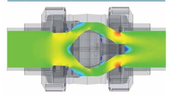
The Type 562 Cone Check Valves are designed for both vertical and horizontal applications. A spring is seated between the cone and the guide to allow the valve to properly seal in applications where a traditional ball check valve would not.
