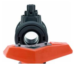
The Type 546Pro Ball Valve seat carrier is reverse threaded while the valve nut utilizes a standard thread. This ensures that the seat carrier is not inadvertently tightened when the valve nut is tightened and avoids possible stem failures.
