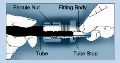
**Caution:** To ensure proper assembly, tubing MUST be fully inserted into the fitting body to the tube stop.
