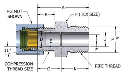
Section shown with Nut Style, **PG**, Plastic Gripper Nut
