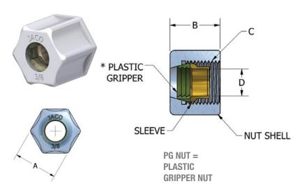
\*Note: P/K Material Nut: Use PVDF Material Gripper, N/C Material Nut: Use Acetal Copolymer Gripper
