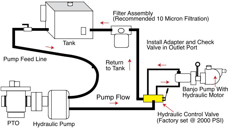
WARNING! DO NOT RUN PUMP DRY, RESTRICT OR REDUCE PORT SIZES OR DEAD HEAD PUMP
