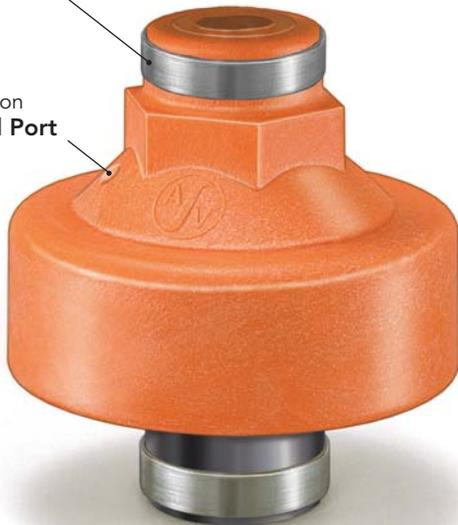
Chemline SG Series Gauge Isolators allow inexpensive pressure gauges, or any other pressure instrument to be used in corrosive services. The upper chamber (gauge side) is filled with a stable fluid such as glycol or glycerine<sup>2</sup>. A diaphragm separates it from the lower chamber which receives the media under pressure.
