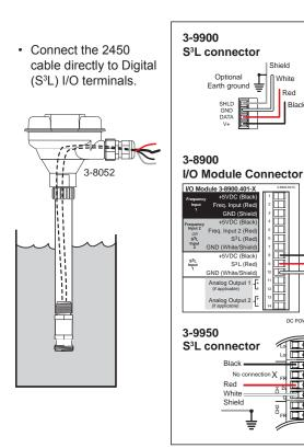
When the 2450 includes a junction box, connect the 2450 terminals to any Digital (S3L) I/O port as shown.
