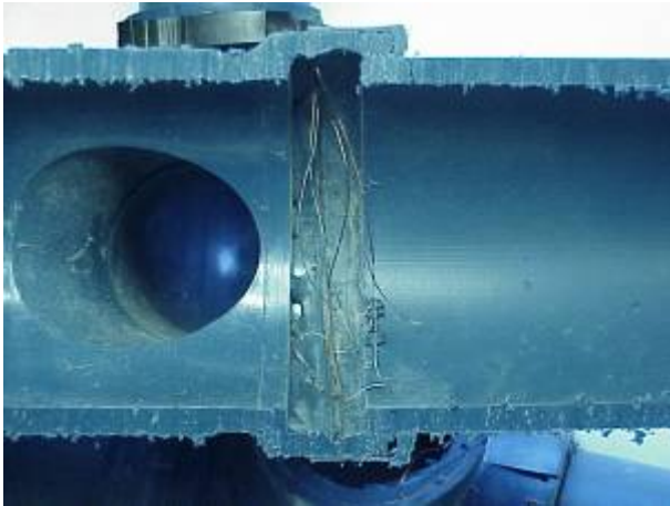
Pipe was not full inserted to the pipe stop!
