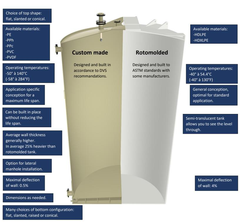
For both types of tank, Les Plastiques Cy-Bo offers the possibility to install connections threaded, flanged, tank adapters and sanitary adapters.
