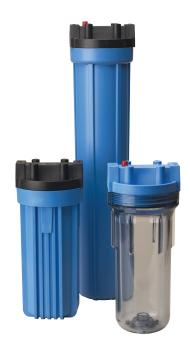
Pentair® Pentek® Standard Filter Housings are manufactured of a durable polypropylene or clear Styrene-Acrylonitrile (SAN). All are equipped with 3/4" NPT inlet and outlet ports. Standard Filter Housings are available in both 10" and 20" lengths and will accommodate a wide range of 2-1/2" to 2-7/8" diameter cartridges. The reinforced polypropylene cap offers an optional pressure-relief button on the inlet side to relieve pressure inside the housing when changing filter cartridges.
